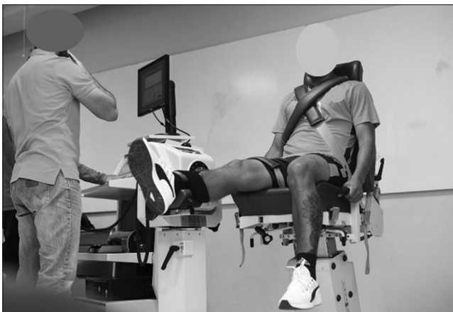
Figure 1. Measurement of the IPKJ in the Biodex® Isokinetic Dynamometer
