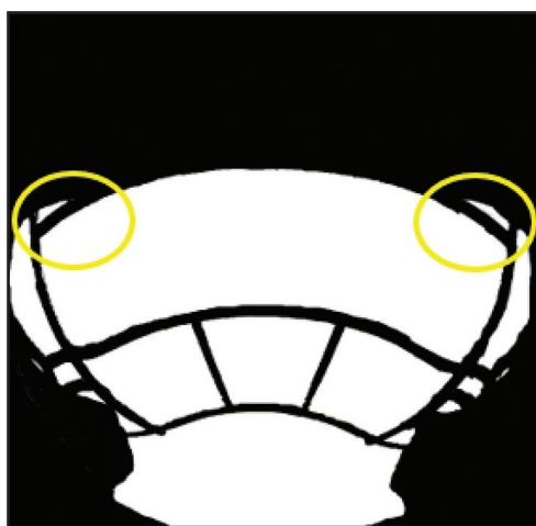
Figure 7. SpeedFlex blockage, black and white edited image (with circled areas indicating potential points of peripheral blockage as compared to the modified helmet)
